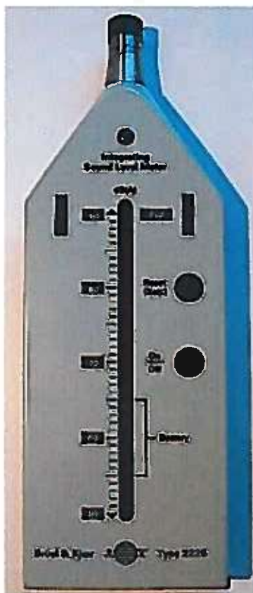
A sound level meter , a basic tool in measuring sound.
